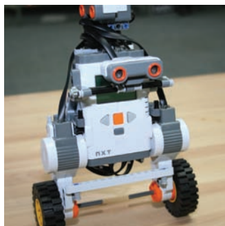
"Segway style" controller, to balance, move and steer: designed and built by Byl's graduate students: Giulia Piovani (ME) and Pat Terry (ECE)
