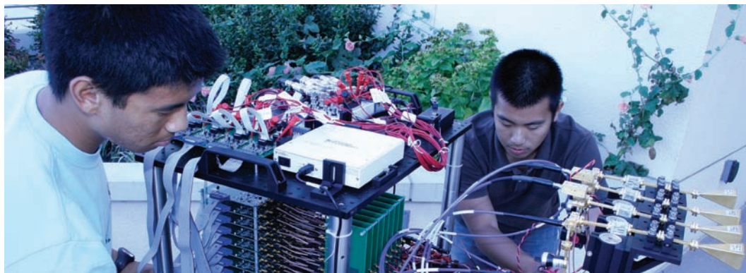
Pictured: Chris Chan and Alvin Fong (above); Eric Torkildson and Hong Zhang (cover photo). Shown is a 60 GHz MIMO prototype (built by Colin Sheldon, Munkyo Seo and Eric Torkildson) that has been used to demonstrate that spatial multiplexing (sending parallel data streams over the same band) is possible even in line of sight environments.
